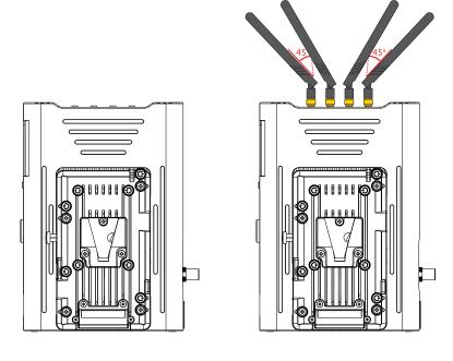
2. Please place the receiver at a height of around 1.5 to 2 meters above floor.
