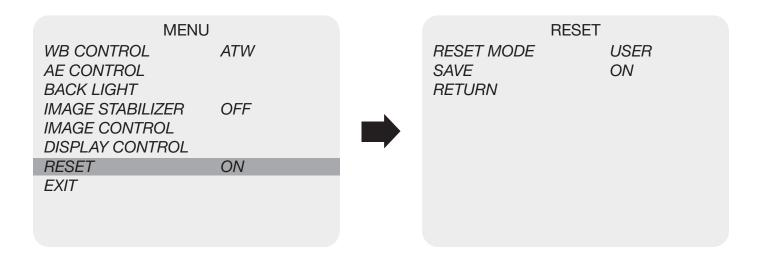
• **ON:** Set the camera reset setting to either FACTORY or USER saved settings which is defined from CHANGE menu.
