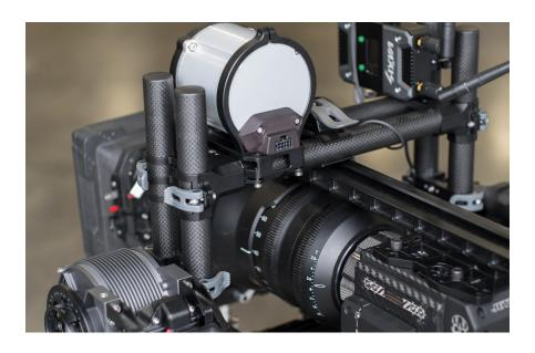
Reinstall the lower tube clamps to secure the FOG. Tighten the 4X inner M4x10mm bolts (shown in red) before tightening the 4X outer bolts. Use Loctite 243 if the FOG will be permanently attached to the MōVI XL.
