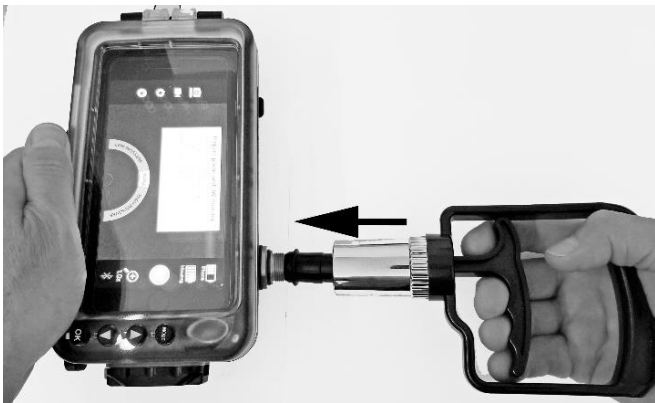
Hand pump pressed against vacuum check port
